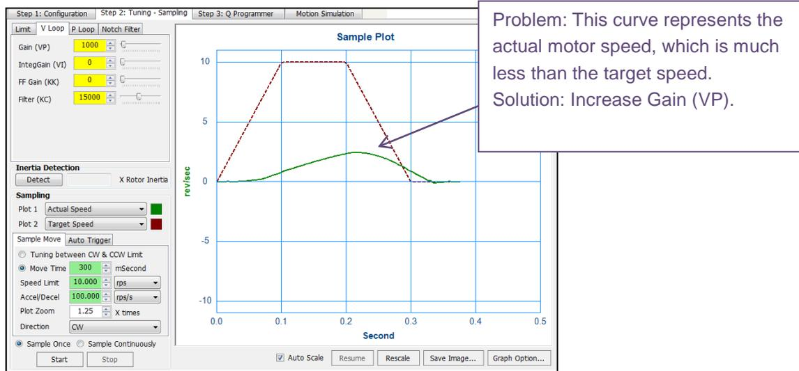
**Figure 6.3.2a:** Sample move with Actual vs. Target Speed plotted
