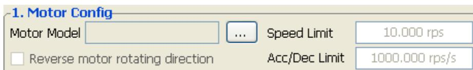
Click "...”to activate the Motor Setup dialog. In this window maximum current, speed limit, and accel/decel limit can be set.
